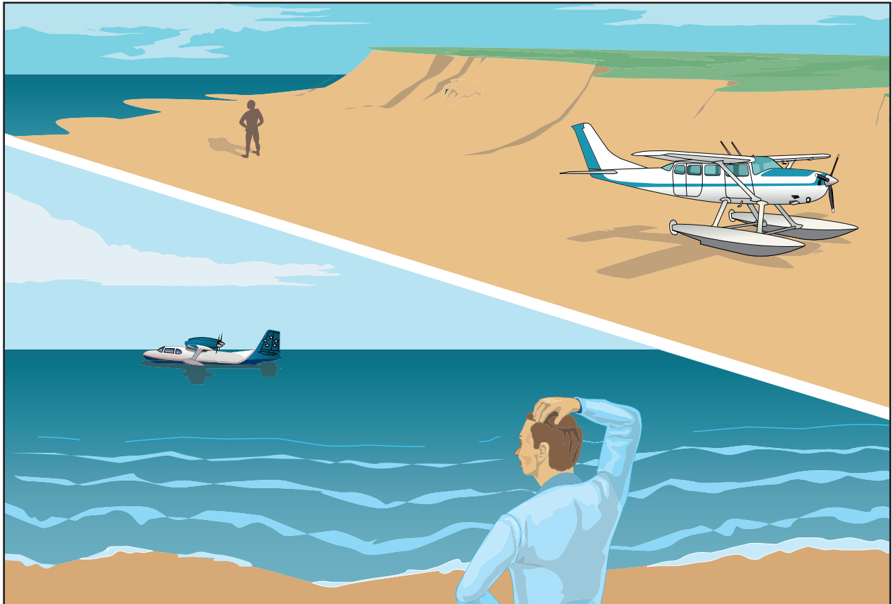
Figure 3-2. An outgoing tide can leave a seaplane far from the water. A rising tide can cause a beached seaplane to float away.
